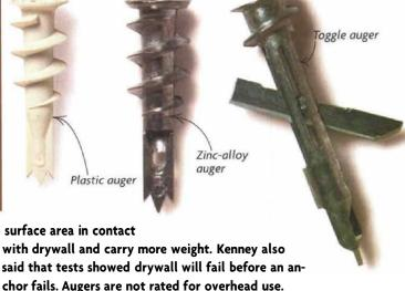
Cobra Anchors and ITW/Buildex both make a combination toggle auger (photo above right). After the anchor is screwed into the wall, a machine screw driven into the anchor flips a toggle over, securing it against the back of the wall. In  $V_2$ -in. drywall, it has a tensile capacity of 20 lb. to 30 lb. and a shear capacity of 50 lb. to 60 lb., and can be used to hang mirrors, picture frames and small cabinets. They cost about \$1.75 for a package of two.
